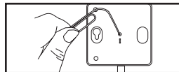
Figure B3 - Press and release the recessed button on the bottom of the bridge
